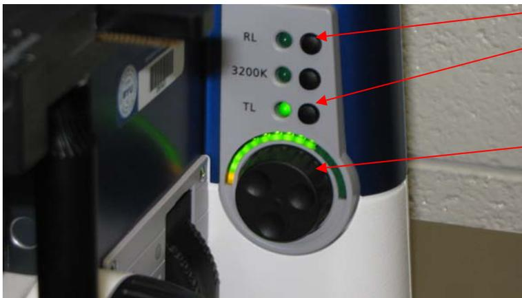
This knob controls the amount of light you will see. The light wheel above the knob shows what level of light is allowed to pass through the microscope.
